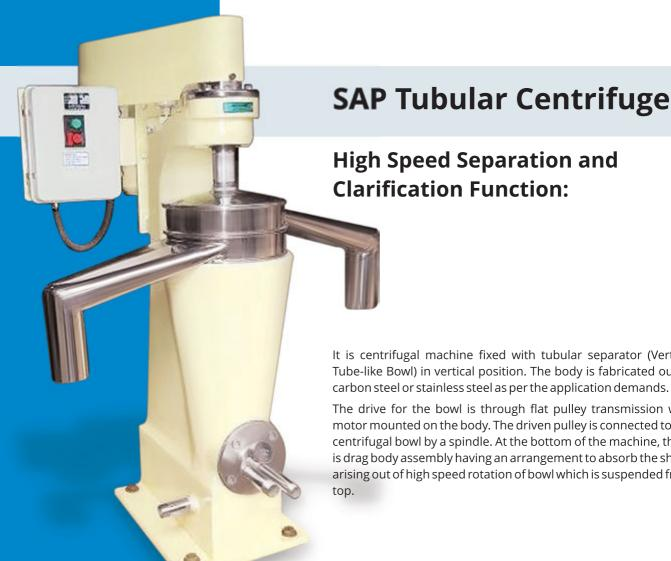
It is centrifugal machine fixed with tubular separator (Vertical Tube-like Bowl) in vertical position. The body is fabricated out of
